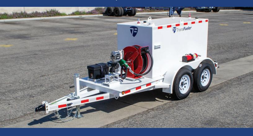
This package includes a 500-gallon double-wall tank with a carbon steel primary tank and internal baffles. The outer containment is made of mild steel with a powder-coated finish. It's mounted on a 7K GVW double-axle steel trailer, DOT-approved for diesel fuel, and can be towed on public roads when full.
